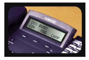
In this example the calling party has called extension 203, which is engaged. The display on their phone then gives the choice of either, CBK (a Call-Back), MSG (Leave a MeSsaGe) or CAMP (Camp-on, used mostly when trying to put an incoming call through to an engaged extension. The incoming call is camped onto the engaged extension, as soon as they finish the current call, the waiting call is automatically put through. Recall timers etc would normally still apply).
